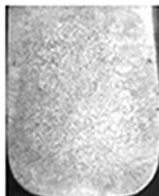
Figure 10 The final solidification structures of Al-4.5% (mass) Cu alloy in water-cooling Cu mould.
